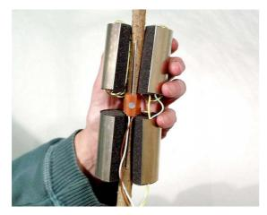
Put the heater and compensating part over the thermosensor assembly. Watch the needle to avoid the direct contact with heating elements (yellow pipe)
