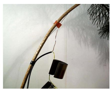
Choose the right place on the branch or stem, remove dry rests of bark from the surface (just by hand), tape the cable and place the temperature sensor assembly.
