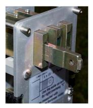
The electrodes should not be inserted completely, a part of ram should remains outside according to overhang value calculated from the formula written on the frame label. Use a rough scale on ram - the accuracy is not the most important topic here.
