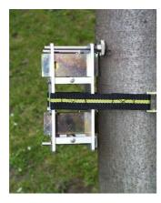
The guide frame should be parallel with the bark surface. Than, push the guides in touch with bark by finger.
