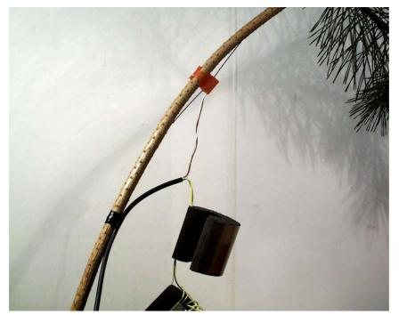
Choose the right place on the branch or stem, remove dry rests of bark from the surface (just by hand), tape the cable and place the temperature sensor assembly.
