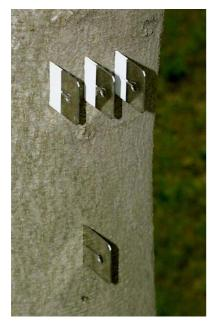
The measuring point after removing of tool looks like this. The visible length of white insulated part depends on the measured value of bark+phloem thickness.
