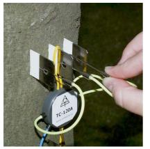
Finally, the weather shield should be fastened.
