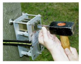
First of all, the bark+phloem thickness has to be measured. Use the longer stick with a plate on its end. Hammer it gently inside until you feel that the
