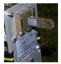
wood has been reached. Also the sound will change at that moment. Read the value on the scale and calculate the "overhang". See label on the tool upper plate.
