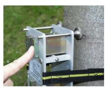
Now, the tool is ready for hammering of electrodes.
