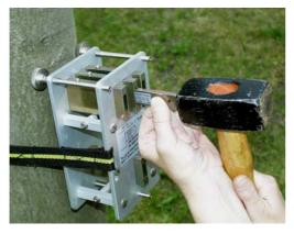
First of all, the bark+phloem thickness has to be measured. Use the longer stick with a plate on its end. Hammer it gently inside until you feel that the
