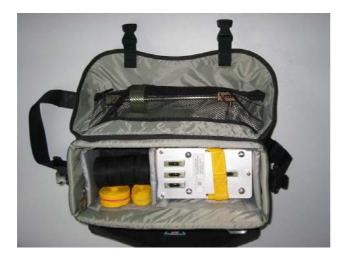
This assembly keeps the guides for proper (= parallel) inserting of electrodes. It must be well fastened with the strap and leveled with rectification bolts.
