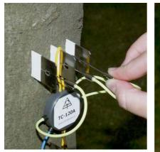
Finally, the weather shield should be fastened.
