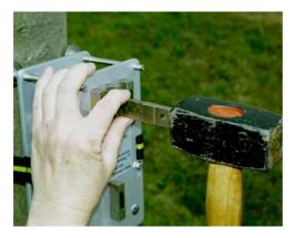
Hammering of electrodes needs some basic skills is order to avoid shifting of the tool assembly. Otherwise the electrodes will not be as parallel as they should be.
