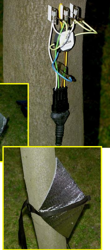
Please be aware that the measurement can be affected by irradiation of the stem below the measuring point when the slightly warmed sap is passing through the artificially heated space. Therefore, especially by solitary trees, it is necessary to shield the sensitive part of stem. Use the skirt placed over the weather shield according to following pictures. Do not fasten the skirt close to stem; let an air gap between them
