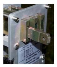
The electrodes should not be inserted completely, a part of ram should remains outside according to overhang value calculated from the formula written on the frame label. Use a rough scale on ram - accuracy is not the most important issue here.
