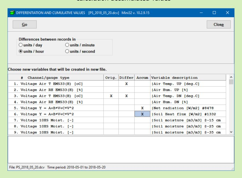
"Export" submenu – Time shift – correction of wrongly set data acquisition time (with resolution of time span between lines)
