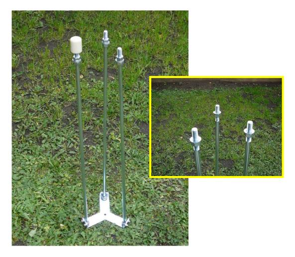
Put the three-arm plate on pins and screw-up upper nuts with washers. In case of need fasten the datalogger assembly to the plate with two M4 screws. Keep roughly horizontal level of the plate:
