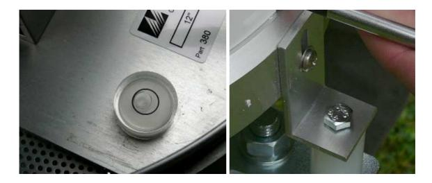
or by means of both big nuts on each pin (new rain gauge miss a leveling system):
