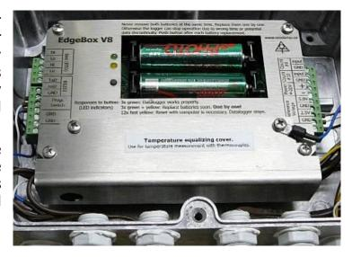
In the upper panel, there is an opening for battery holders. Here are also two LED diodes and a check button for brief system test.
