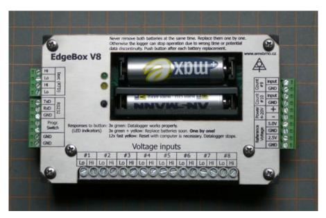
Note: The temperature measurement with RTD thermosensors supposes four-wire connection. Two wires lead the excitation current (ca 150  $\mu$ A) to the sensor and next two wires connect the sensor voltage to measuring terminals. Excitation wires should be connected to terminals labeled as Iexc (RTD).
