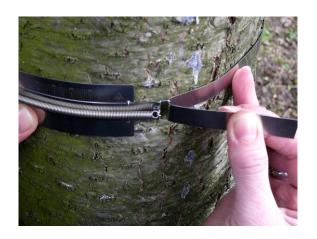
6/ Watch the scale – the correct position is a few millimeters behind zero
