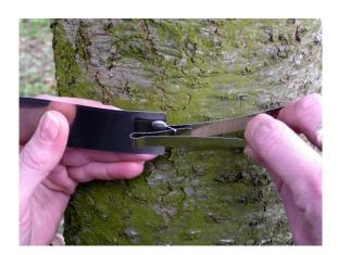
3/ Set the scale to the right position and wrap the tape around the trunk
