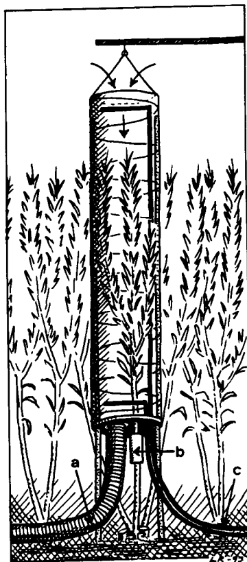
Fig. 1: The design of the chamber and set-up of the measurements: a - tube leading to a ventilator and propeller anemometer; b - THB-device measuring sap flow; c - polyethylene tubes leading to IRGA - air is taken in at the top and bottom of the chamber via perforated segments placed horizontally across the chamber.
