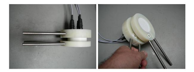
Note 1: Screw back the lid by hand only. Use the tool only for finalizing but with a limited power only!
