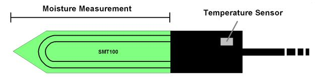
Figure 2: Sensor SMT100 with green capacitive measurement field and position of temperature sensor
