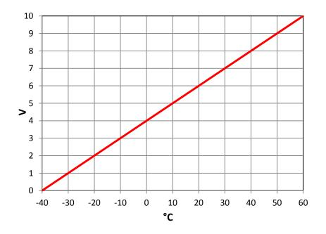
Equation for calculating the temperature T from the measured output voltage U: T [°C] = (U - 4.0) \* 10 Example: U = 6.5 Volt  $\rightarrow$  T [°C] = (6.5 - 4.0) \* 10 = 25 °C
