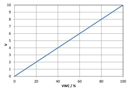
Output voltage [V] versus soil moisture [VWC] for standard version 0-10 V:
