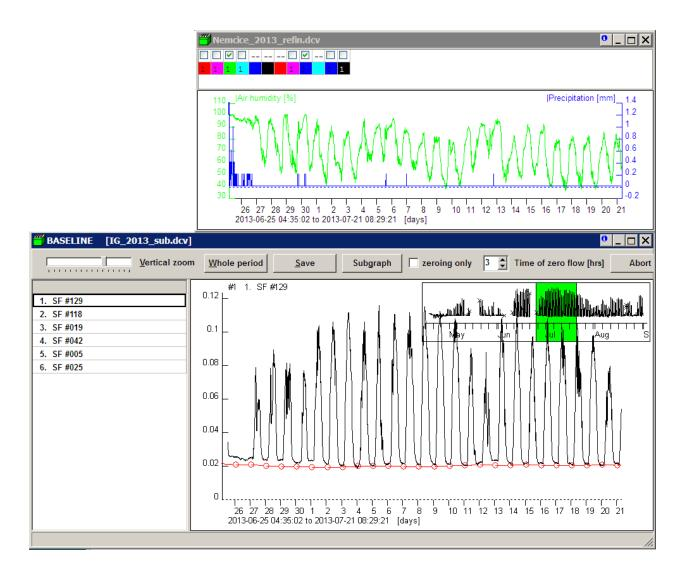
The air humidity and precipitation variables were selected in the upper window. There are only a few nights with high air humidity and also only four rainy events with the 0.2 mm of precipitation only. The baseline created with respect to those weather conditions for selected subperiod of time is shown.
