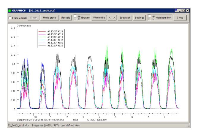
Baseline business is the trickiest part of data processing. The HB method working with low value of temperature difference (in order to save energy) is sensitive to external disturbing factors (like ambient temperature gradients, temperature inhomogeneities inside the measuring points etc.) under very low water movement.
