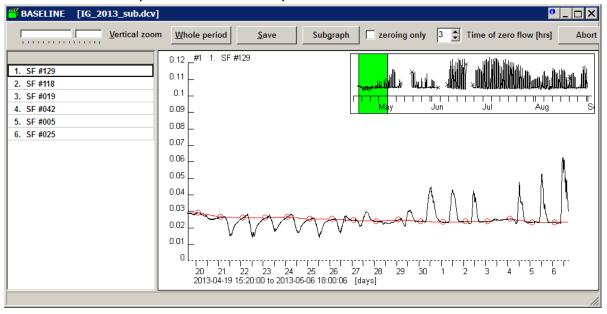
Typical situation at the beginning of growing season: European beech after the bud break. The strange pattern in days with 'negative' sap flow values can be explained by high vertical temperature gradient within the stem or outside. The system reduced power because this gradient helped to reach set temperature difference. The situation improved with the first leaves – the water stream 'smoothes' disturbing gradients.
