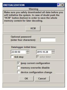
Initialization ('Init') deletes whole memory content and offers some important possibilities like datalogger time setting, ('Set time' option available at any time has certain limits in setting time backwards) changing the memory operating mode (memory overwrite), returning to original (intact) factory setting and changing the mode of operation of the unit from standard to advanced and vice versa.
