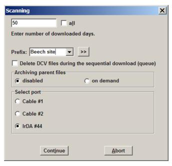
In sequential mode, the computer is continuously searching sensors. If it establishes connection, it immediately downloads the preset amount of data (in days) and saves them in file.
