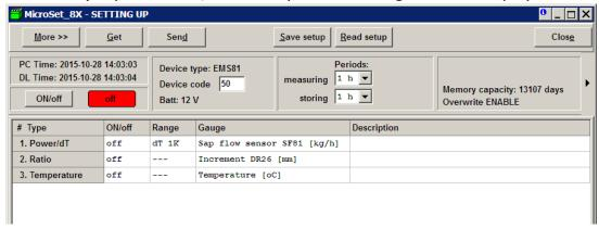
The screen shows computer time (clock time) and time of datalogger. Note that the datalogger time should be always solar time – Mini32 sets during initialization always solar time according to local computer setting independently on the season.
