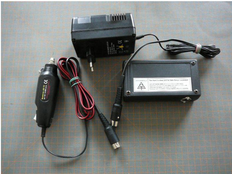
It consists of the drill, battery box with electronics and battery charger. The drill keeps low revolutions until it faces a hard xylem. Then, it increases the power until the drilling resistance gets low again. The recommended drill bit diameters ranges between 0.8 to 1.0 millimeters. Proper bits should be chosen according to xylem properties. Principally, the smaller hole the better.
