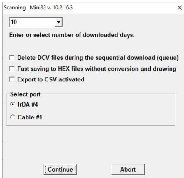
In sequential mode, the computer is continuously searching for sensors. If it establishes connection, it immediately downloads the preset amount of data (in days, max 999) and saves them to file.
