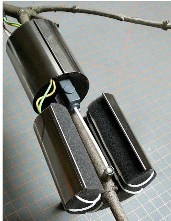
The installation of measuring point is fast and easy. Just a special drill is necessary for drilling holes for needles in xyloid stems.
