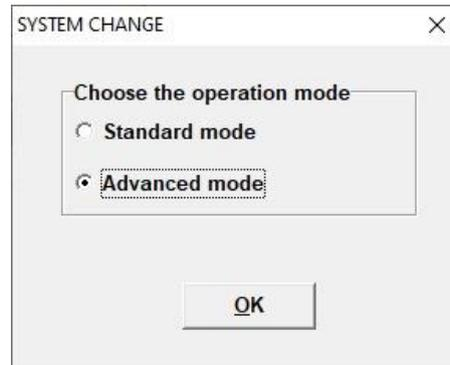
Advanced mode of operation expands the number of recorded variables for those interested in the measurement details. In this mode user can log temperature difference in behind the heater, power supply voltage and error status during the measurement:
