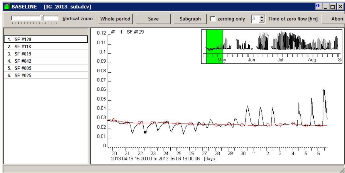
Typical situation at the beginning of growing season: European beech after the bud break. The strange pattern in days with 'negative' sap flow values can be explained by high vertical temperature gradient within the stem or outside. The system reduced power because this gradient helped to reach set temperature difference. The situation improved with the first leaves – the water stream 'smoothes' disturbing gradients.
