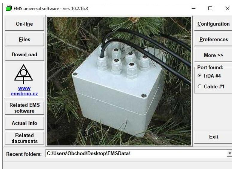
Connect the IrDA/USB data cable. Make sure that the information about the cable port appears on the right side of the Mini32 main screen. Otherwise install the USB driver from the installation package (push "Related EMS software" button).
