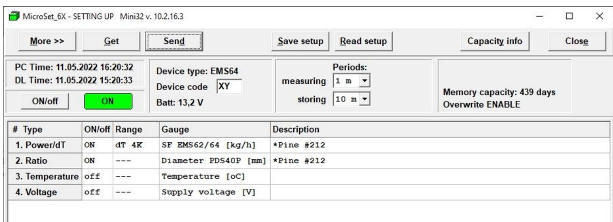
System is on. The voltage 13.2 V shows good battery status. Device code (alphanumeric code, unfortunately two characters only due to compatibility with older systems) is set by user.
