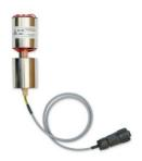
of heating elements (in direction of water movement). Second cylinder has no heater and it just covers the reference needle thermocouple located with respect to he thermal symmetry. The water passing along the sensor is warmed and the heating power is controlled in order to keep the temperature difference between needles. Then, the input power is directly proportional to the amount of water passing the sensor in terms of kg/hr.
