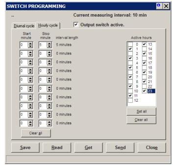
This example shows configuration for switching on the GSM modem every other hour for five minutes. Note, up to ten independent time intervals can be set within one hour.
