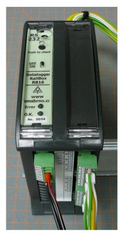
The battery and system status are indicated by two LEDs on the upper panel. The green LED indicates normal operation. During the regular measurement it is on as well as when communicating with PC or other external system (modem).
