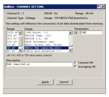
EMS12 is the sensor measuring the photosynthetic active radiation.
