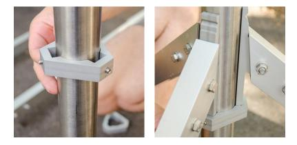
Put on the upper sleeve and fix the leg assembly to the central tube. Set the right position on the tube according to demanded height of sensor above the ground and tighten all six hexagon socket set screws.
