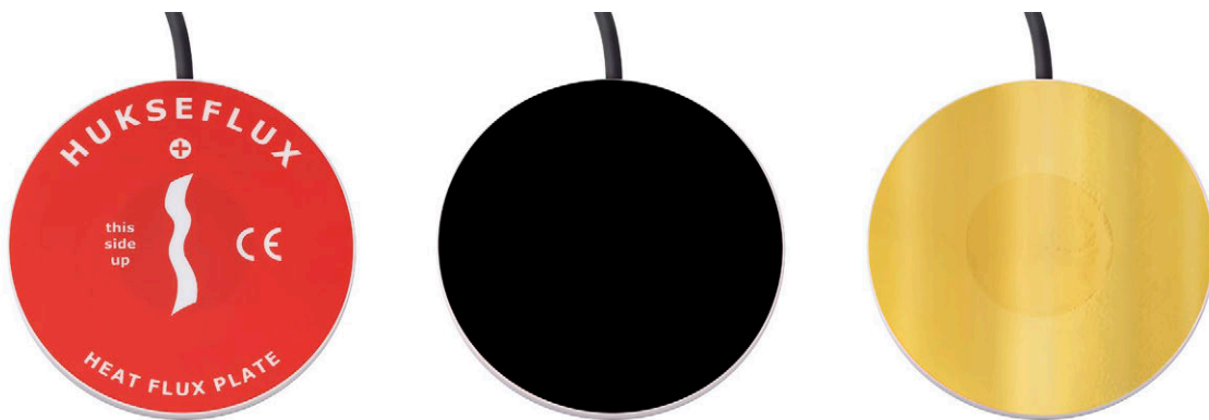
Figure 0.3 HFP01 heat flux plate: with BLK-80 and GLD-80 stickers to measure radiative and convective heat fluxes separately
