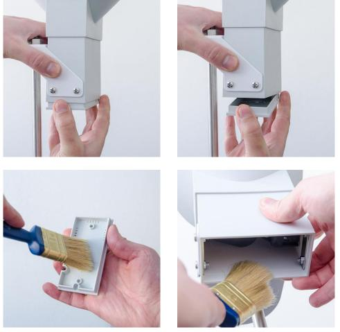
After cleaning, put the funnel on and insert the sieve. Check the horizontality of the rain gauge, resp. verticality of the support pin.
