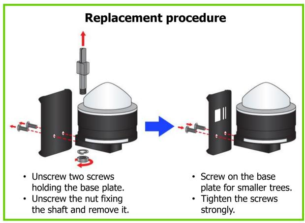
Keep in mind that different types of screws may have been used - use the correct one according to the hole in base plate (supplied with the base plate).
