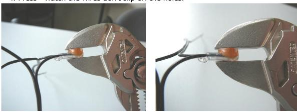
Note that the orange head is fully inserted and does not overlap the transparent clip body. Also note the silicon outflow out of the clip.
