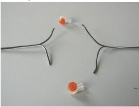
2. Insert wires inside the clip holes. To the end!
