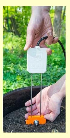
For more comfortable work you can remove inserting guide tool in half of rods length.
