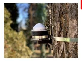
Dendrometer measures variations of the stem diameter (SDV) with high spatial (micrometre) and temporal frequency (hours). The pattern of SDV is based on (1) irreversible stem growth dynamic and (2) tree water regime.
